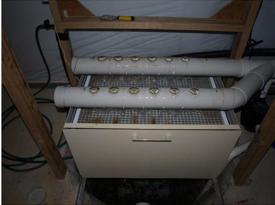
Figure 2: A static screen filter showing the delivery manifold (to utilise as much of the screen area as possible) and removable filter screens.
