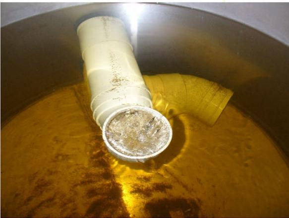
Figure 1: A swirl sedimentation tank showing the tangential inlet (bottom of the tank) and the solids being directed to the centre bottom of the tank. The outlet is at the water surface or centre of the picture.
