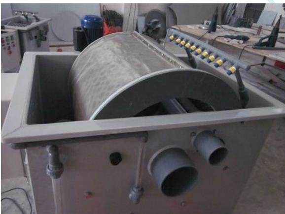
Figure 3: A drum screen filter showing the series of high pressure spray nozzles for the back flushing procedure. ([http://china-aquaculture.en.alibaba.com/product/501875208-210823815/Rotary\\_Drum\\_Filter\\_fish\\_farm\\_aquaculture\\_equipment.html](http://china-aquaculture.en.alibaba.com/product/501875208-210823815/Rotary_Drum_Filter_fish_farm_aquaculture_equipment.html)).
