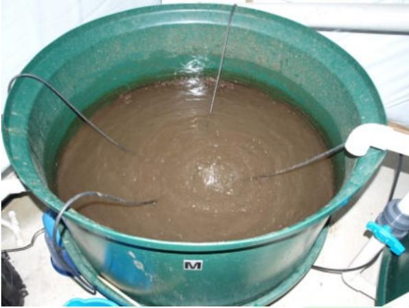
Figure 5: A simple “off line” solids mineralisation tank showing aeration. The pipe and valve at the right is the solids drain from the sedimentation tank to the mineralisation tank.
